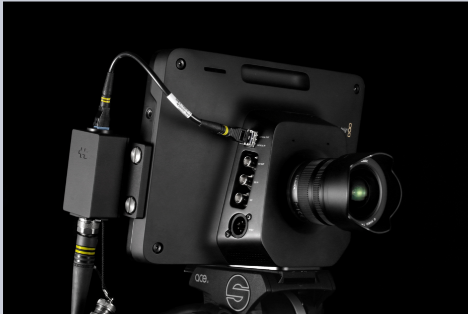
A completely installed Adapter Two with FieldCast main cable on the one side and LC bridging cable to Studio Camera on the other side.
